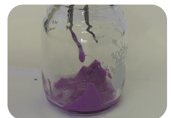
Flexi Dam after one hour immersion dissolved into a formless gel.
